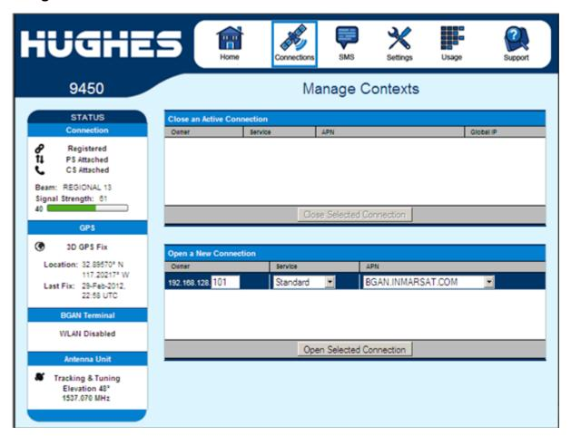
**Manage Connections** page under the Data tab allows the user to setup and configure PDP contexts (data connection) for any TE that is connected to the UT. It also shows you all current Active Connections.
