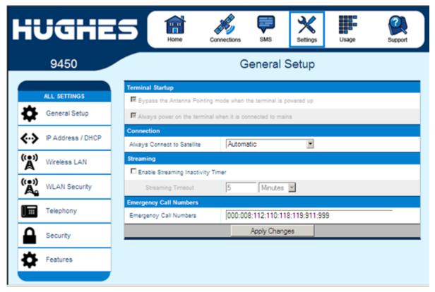
**Streaming** – By enabling this parameter, the user can turn on a timer for inactivity for a streaming QoS that has been set up. The timer is in either seconds or minutes and will tear down a streaming context after  $\mathbf{X}$  seconds or minutes of inactivity.
