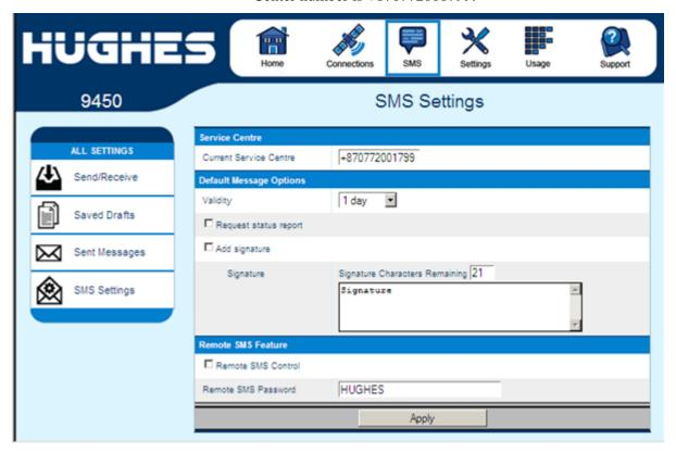
On the **Remote SMS Feature** section you can enable the unit to receive and act on special remote control SMS messages. Contact your service provider for more information on this feature. Before this feature can be enabled you must obtain the feature activation code from your service provider and activate the feature from the Features Web page.
