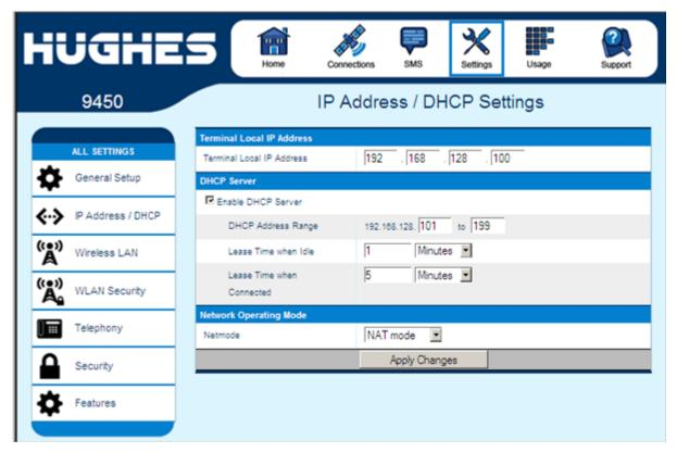
**DHCP Server**: allows the DHCP server in the UT to be turned on or off by checking the Enable box.
